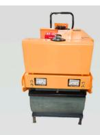
• JP Engineering Services Which is engaged in presenting a walk behind Double Drum Vibratory Roller is modern compact design for use in a wide range of compaction application. Hydraulic with integrated travel control eases the operating efforts required for movement.
