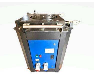
• A **Bar Bending Machine** is a piece of equipment used in construction and manufacturing to bend metal bars, typically reinforcing bars (rebar) used in concrete structures. These machines are essential for shaping rebar to specific angles and curves as required in various construction projects, such as buildings, bridges, and other infrastructures.
