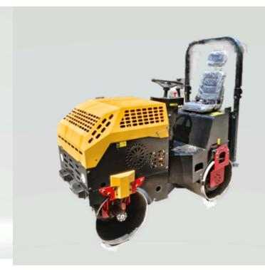
• We are offering a wide assortment of Hydrostatic Roller, Which is Designed for finish layers of asphalt as well as granular sub base material in confined areas. Apart from this, this is ideal for Parking lots, Drive way and Shoulder Work. These Product are offered to the clients at very affordable and reasonable rates with in committed periods of time.
